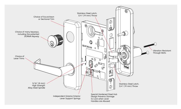
These premium performance locksets are built with a heavyduty mortise chassis for all applications where ANSI/BHMA A156.13 Grade 1 products are required. To meet the aesthetic needs of your project, these versatile locks are available in a range of lever designs and finishes.
